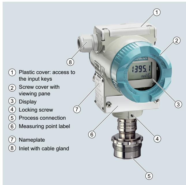
Device front view, SITRANS P DS III
